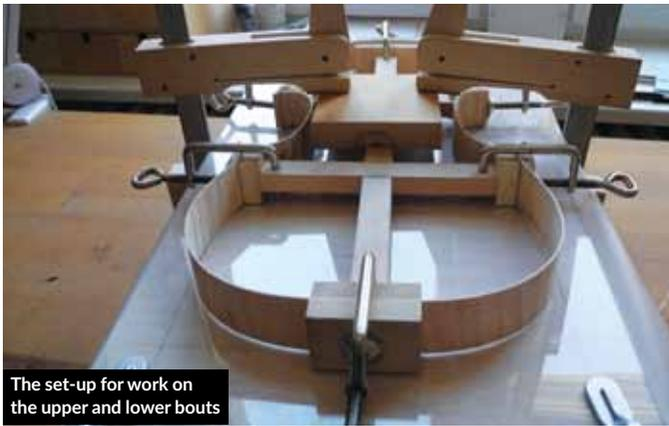
The set-up for work on the upper and lower bouts
