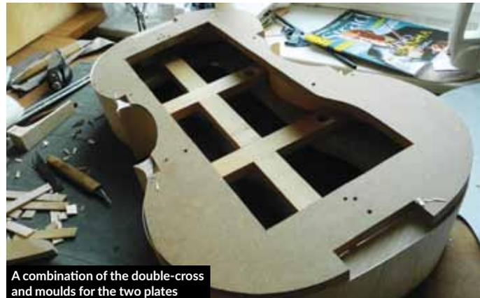
A combination of the double-cross and moulds for the two plates
