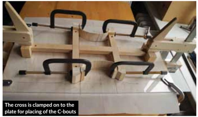
The cross is clamped on to the plate for placing of the C-bouts
